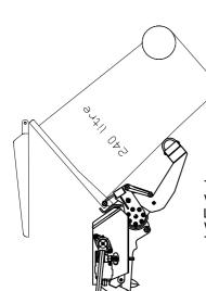
THE ML450 IS HEIGHT ADJUSTABLE, WHICH MEANS IT IS POSSIBLE TO LIFT THE COMMON 240 LITRE WHEELIE BINS AND THE TALLER 600 TO 1100 LITRE FOUR WHEELED BINS
